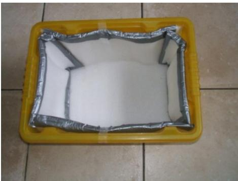
First you need to line the inside of the box with insulation. Cut your materials to size so you have pieces to fit the base, and sides. Single pieces need to be about 1cm thick, so if you are using a thinner material you can make a thicker layer by putting several pieces on top of
