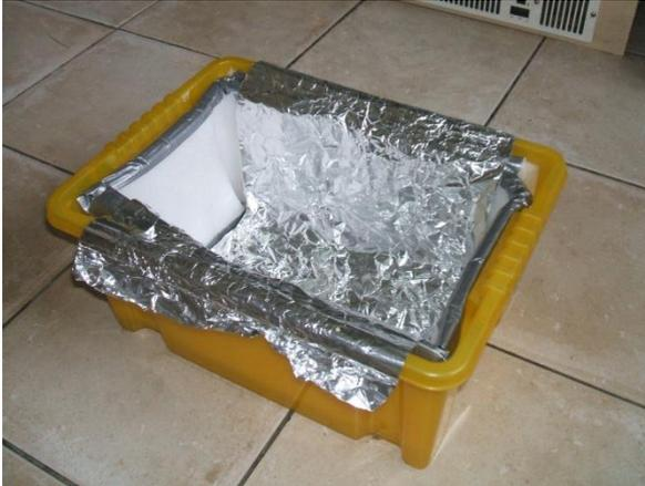
Next line the whole thing with foil. This is to reflect back as much radiation as possible within the extractor.
